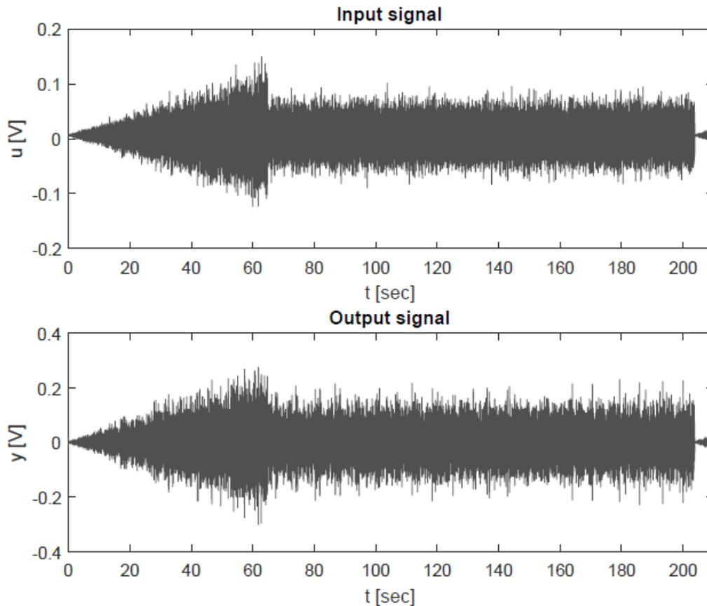
Fig. 2. Available input and output benchmark signals.
