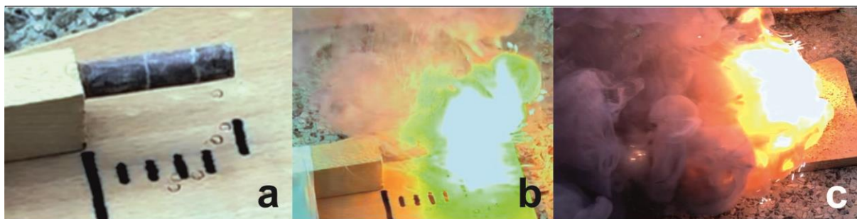
Figure 11. Fuel sample with a diameter of \varnothing 11 mm (a); combustion at atmospheric pressure (b); violet colored smoke (c).
