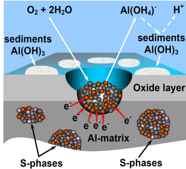
Figure 2. Second (electrochemical) stage of corrosion of S-phase
