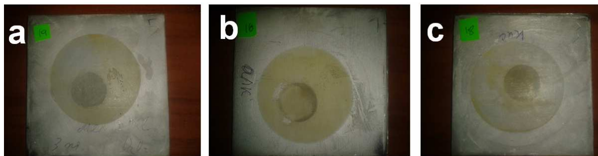
Fig. 24. Samples with CeCC films after different approaches of preliminary treatments, and posterior electrochemical measurements
