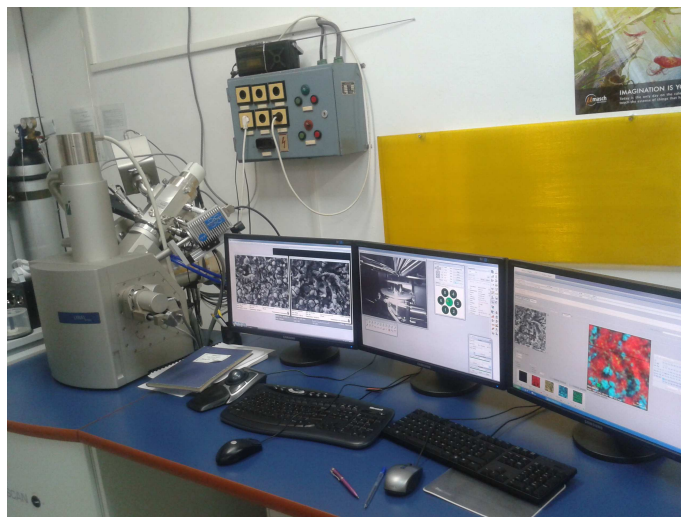
Figure 23. Exterior view of a SEM-EDX device
